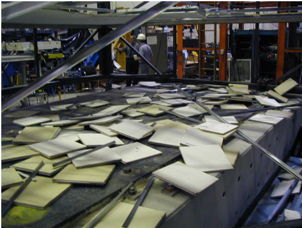
Figure 3–13. Collapse of ceiling system CS3 after 2.5g earthquake excitation.
